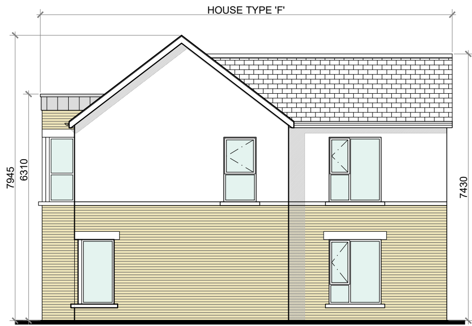
SIDE (DUAL FRONTAGE) ELEVATION @ 1:100 TERRACE BLOCK TYPE 17
